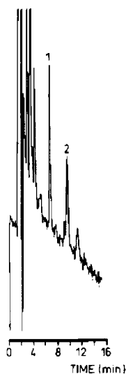
Fig. 2. Representative HPLC chromatogram of 200 \mu l BAL fluid of a patient receiving twice daily 500 mg cefuroxime axetil orally. Peaks: (2) cefuroxime, 54 ng/ml (calculated); (1) cephaloridine, internal standard. Column, Symmetry C_{18} ; mobile phase, acetonitrile–0.05 M ammonium phosphate buffer (pH 3.2) (15:85, v/v); flow-rate, 0.8 ml/min; detection wavelength, 280 nm.
